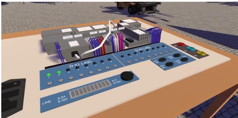
Fig.7. The 3D model of PLC next in virtual environment
