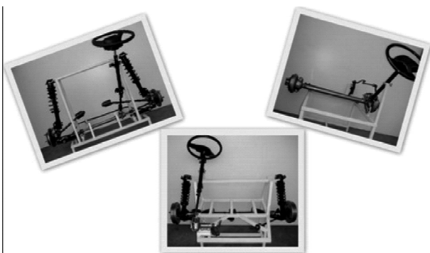
Fig.5 Cut Section Model of Steering System
