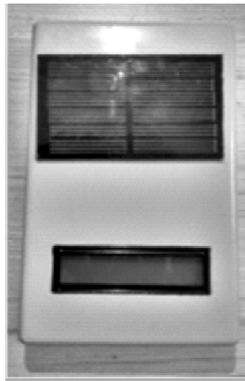
Fig. 5 Solar wireless insolation sensor
