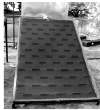
Fig. 7 Solar crop dryer collector
